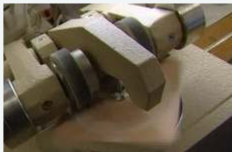
Determination of plywood stability to abrasion (taber-test)
