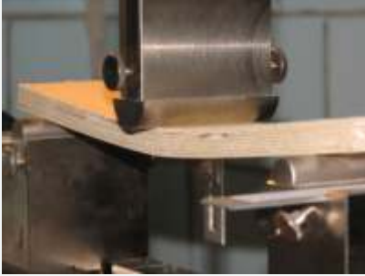
Determination of bending strength of plywood SyPly
