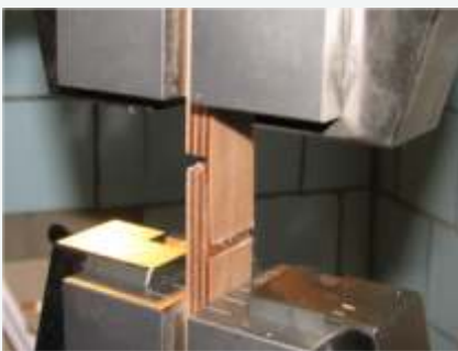
Determination of shear strength on a glutinous layer of plywood SyPly
